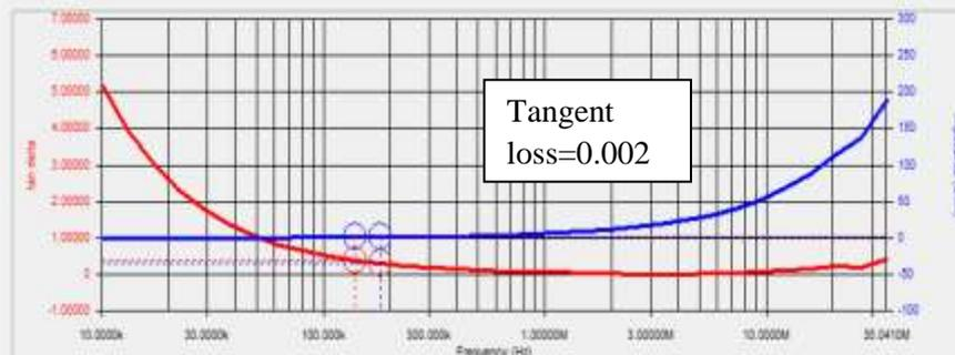
Figure 2: Tangent Loss (N4L)
