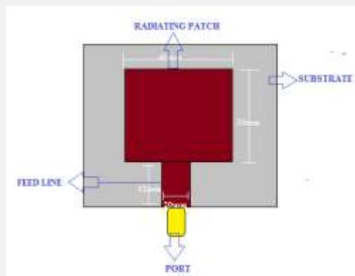
Figure 3: Microstrip Patch Antenna
